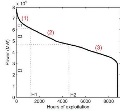
Fig. 2. Example of load duration curve
