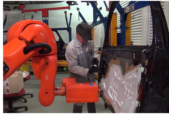
Fig. 2. New assembly task with human-robot co-presence
