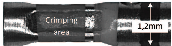
Fig. 9. Contact shape after crimping.
