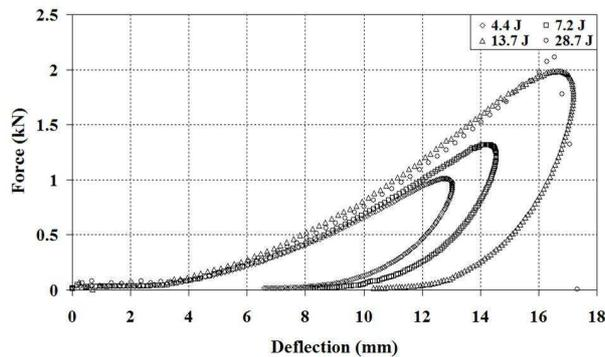
Figure 2. Force-Deflection diagrams for different impact energy levels.
