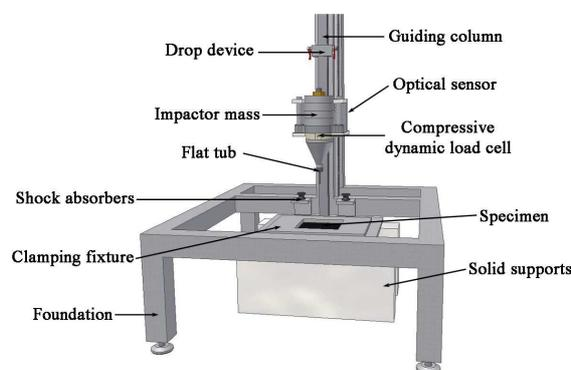
**Figure 1.** Schematic diagram of drop-weight impact testing machine.
