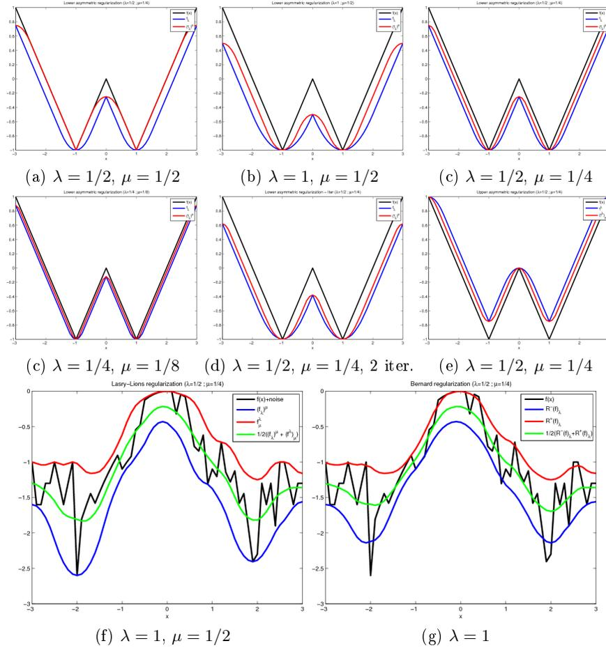
**Fig. 3.** Lasry-Lions regularization of a 1D signal (original signal in black, operator in  $\lambda$  in blue and composed operator in  $\mu$  in red: (a) quadratic opening, (b) to (c) lower regularizer  $(f_\lambda)^\mu$ , (d) iterated lower regularizer, (e) upper regularizer  $(f^\lambda)_\mu$ . Bottom row, comparison between Lasry-Lions regularizers (f) and Bernard regularizers (g). Green curves correspond to the averages.
