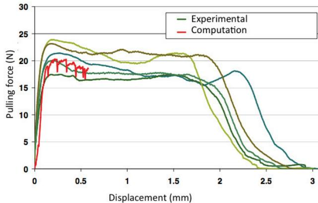
Fig. 7. Comparison of experimental and computational pulling forces.
