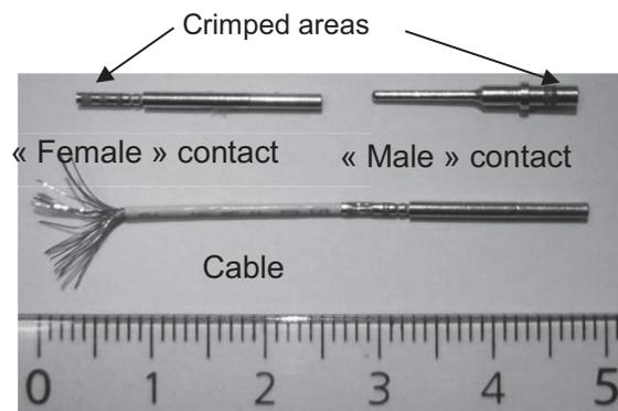
Fig. 1. Size and geometries of the different components.
