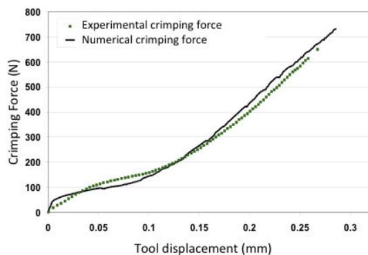
Fig. 5. Comparison of experimental and numerical crimping force.
