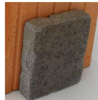
Figure 3: The new aerogel-based coating
