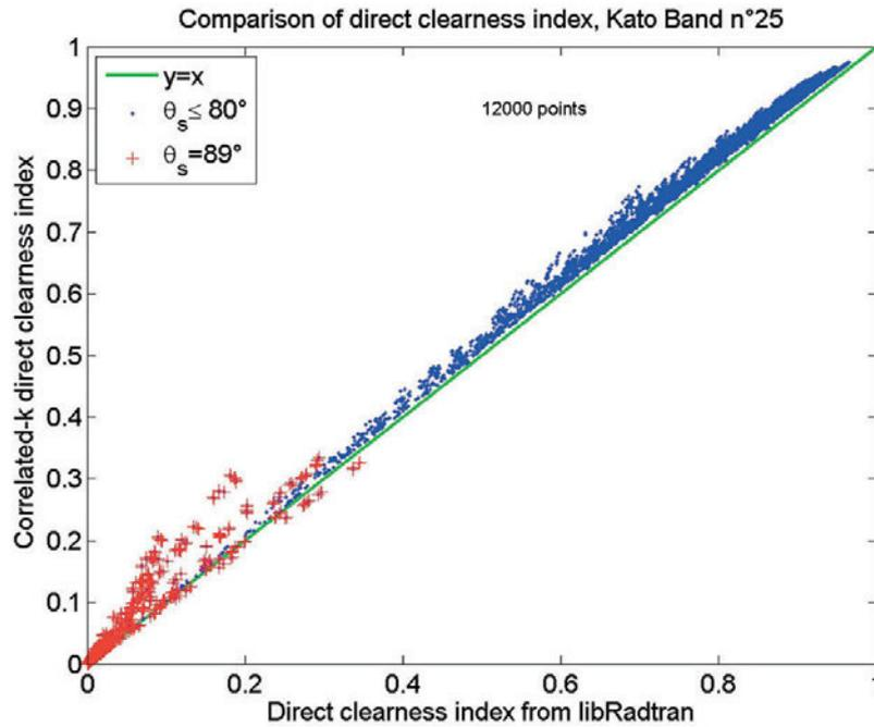
**Figure 5:** Scatterplot between libRadtran spectrally detailed calculations and the correlated- $k$  approximation of Kato et al. (1999) for two ranges of solar zenith angle  $\Theta_s$ . Direct clearness index for KB no. 25 [1516, 1613] nm.
