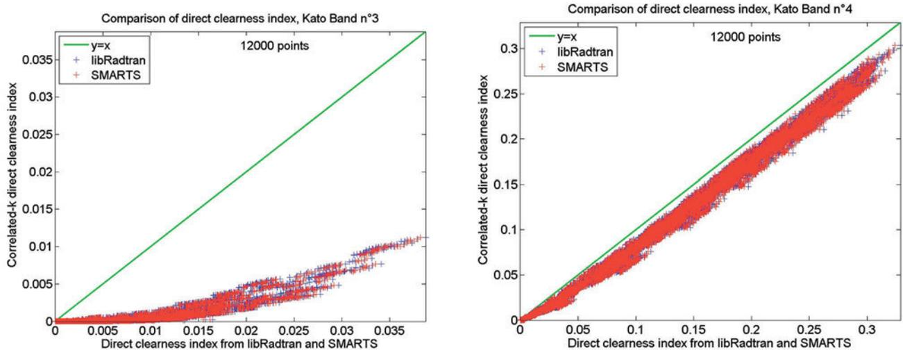
**Figure 3:** Scatterplot between spectrally detailed calculations (horizontal axis libRadtran and SMARTS) and the correlated- $k$  approximation of KATO et al. (1999). Direct clearness index for KB no. 3 [283, 307] nm (left) and no. 4 [307, 328] nm (right).
