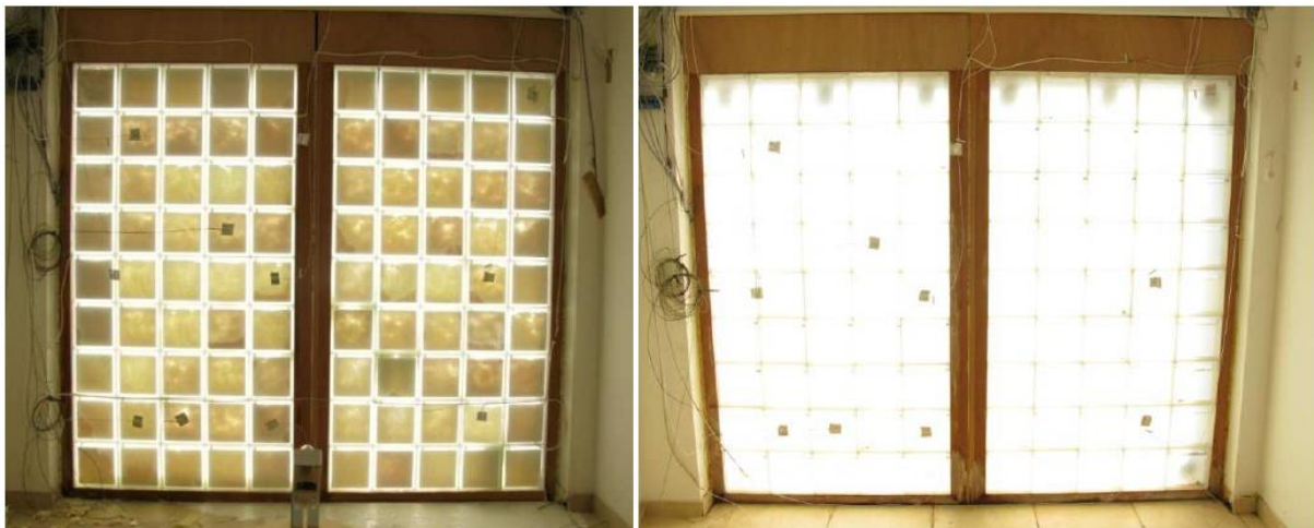
Fig. 6. Daylight provided by the PCM-aerogel wall with the PCM in solid state (left) and liquid state (right). The picture is taken from inside the test room.
