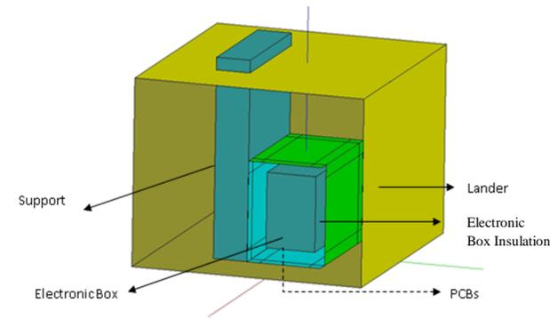
Fig. 14 – AERSUS Instrument Components
