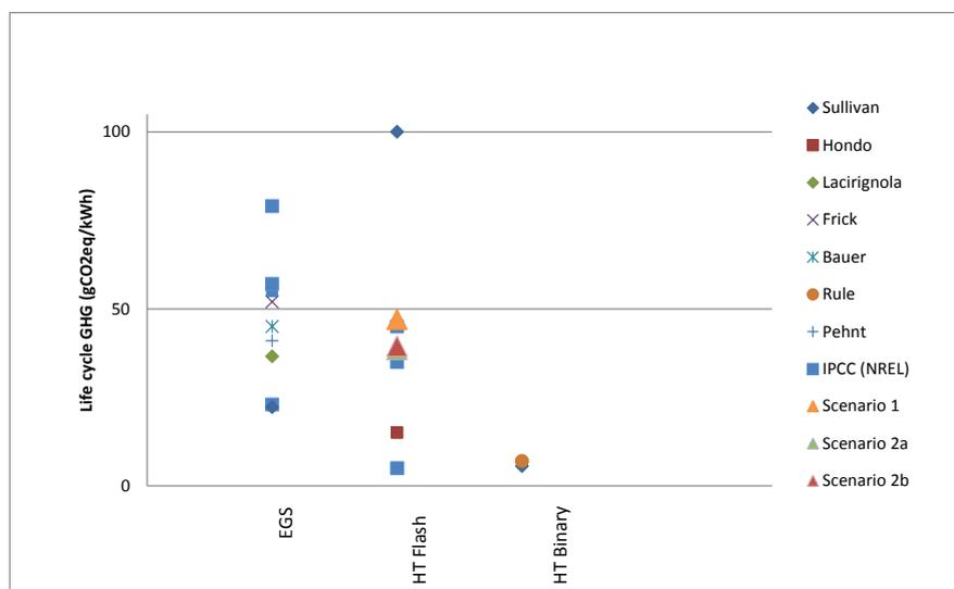
**Figure 3: Comparison of Life cycle GHG associated with geothermal electricity production (in CO<sub>2eq</sub>/kWh), based on a literature survey and considering different technologies**
