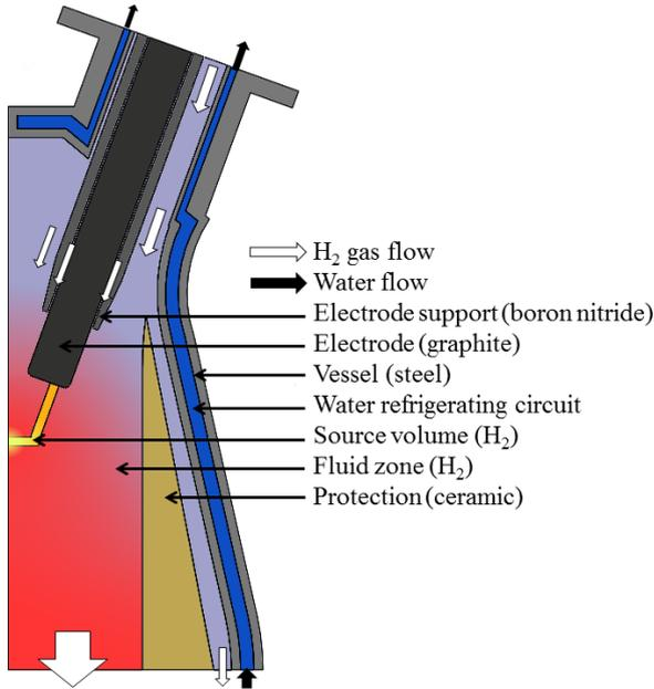
Fig. 2. Sectional view of the plasma torch
