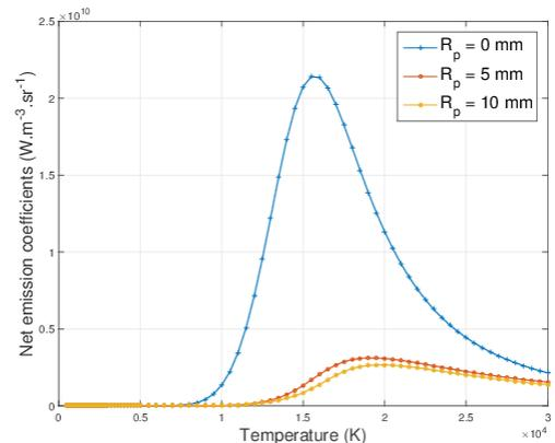
Fig. 1: Net emission coefficient of hydrogen plasma with temperature at 1 bar and for different plasma radii.
