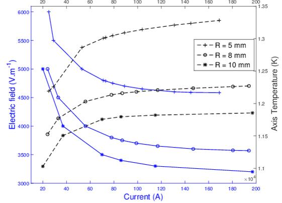
Fig. 6: Electric field and temperature at the axis vs current for a wall stabilized arc column at 20 bar pressure
