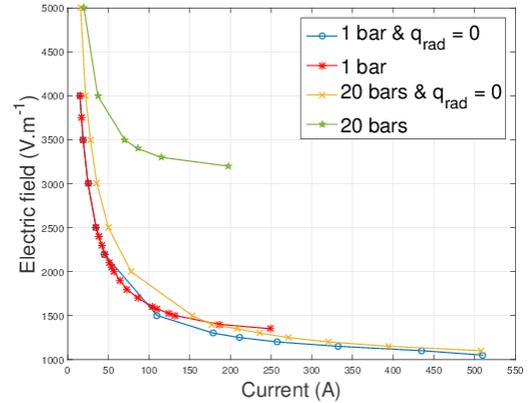
Fig. 3: Current-voltage characteristic of a wall stabilized arc column of 10 mm radius
