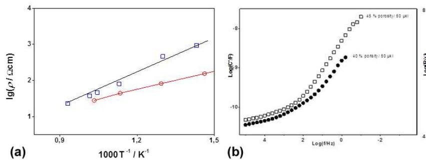
Figure 7. (a) Arrhenius plots resistivity for BCY15 (○) with 12% porosity and YDC15 (□) and (b) frequency dependence of  $C'$  in BCY15 with different porosity and the same pore former.
