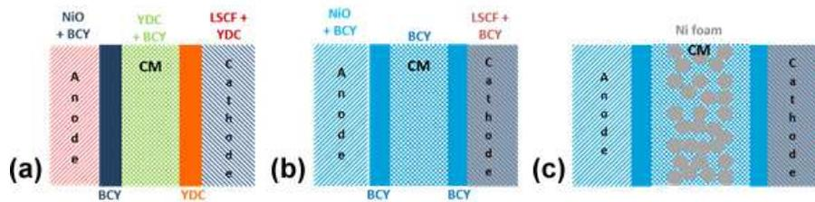
Figure 2. IDEAL Cell evolution; (a) the dual membrane, (b) the monolithic and (c) the nickel foam concepts.
