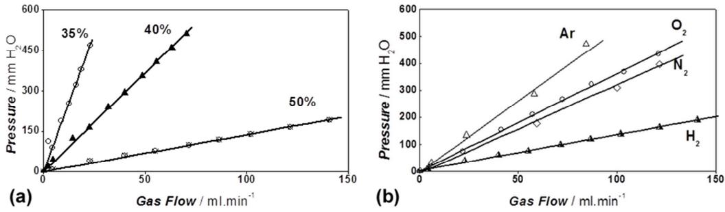
Figure 8. (a) Hydrogen permeability of CMs with different porosity at room temperature and (b) Gases permeability measurements in the CM with 50 vol.% porosity at room temperature.
