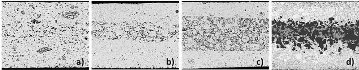
Figure 5. Central membrane porosity sintered at 1400 °C for 5 hours: (a) no-graphite, (b) 10 vol.% graphite, (c) 20 vol.% graphite and (d) 30 vol.% graphite.
