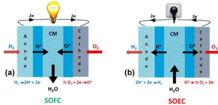
Figure 3. The (a) SOFC and (b) SOEC modes.
