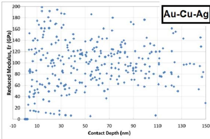
Fig. 2. Example of experimental nanoindentation reduced modulus  $E^*$  results obtained on a *quartier* specimen (rolled and annealed, just before beating, thickness  $\sim 15 \mu\text{m}$ ) of the commercial Au-Cu-Ag alloy.
