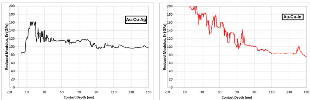
Fig. 3. Statistical trend lines for the reduced modulus  $E^*$  obtained from the experimental nanoindentation on *quartier* specimens (rolled and annealed, just before beating, thickness  $\sim 15 \mu\text{m}$ ) of the Au-Ag-Cu and Au-In-Cu alloys.
