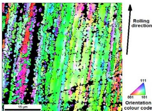
**Fig. 5.** EBSD image on a specimen of the commercial Au-Cu-Ag alloy at an intermediate state of cold rolling (not annealed). The rolling direction and the colour code of crystal orientation are shown beside
