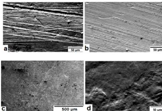
**Fig. 4.** SEM micrographs of the alloys. (a) Au-Cu-Pd at the end of cold rolling; (b) Au-Cu-In at the end of cold rolling; (c) Au-Cu-Ag-In after the first beating (*shoder*); (d) Au-Cu-In after the first beating (*shoder*)
