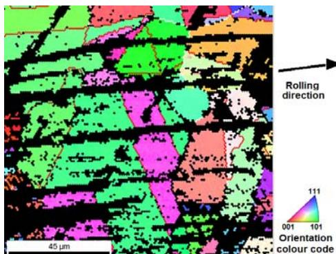
**Fig. 6.** EBSD image on a specimen of the Au-Cu-In alloy after annealing at the end of cold rolling (*quartier*). The rolling direction and the colour code of crystal orientation are shown beside
