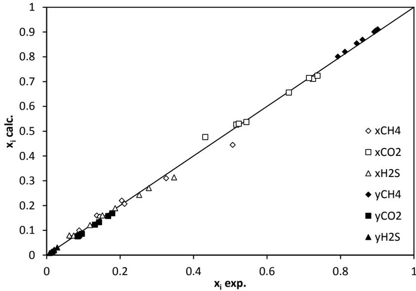
**Figure 9.** Model performances (Yokozeki, 2003 with binary interaction parameters obtained in this work) for the prediction of SLV composition for the ternary CH<sub>4</sub>-CO<sub>2</sub>-H<sub>2</sub>S mixture.
