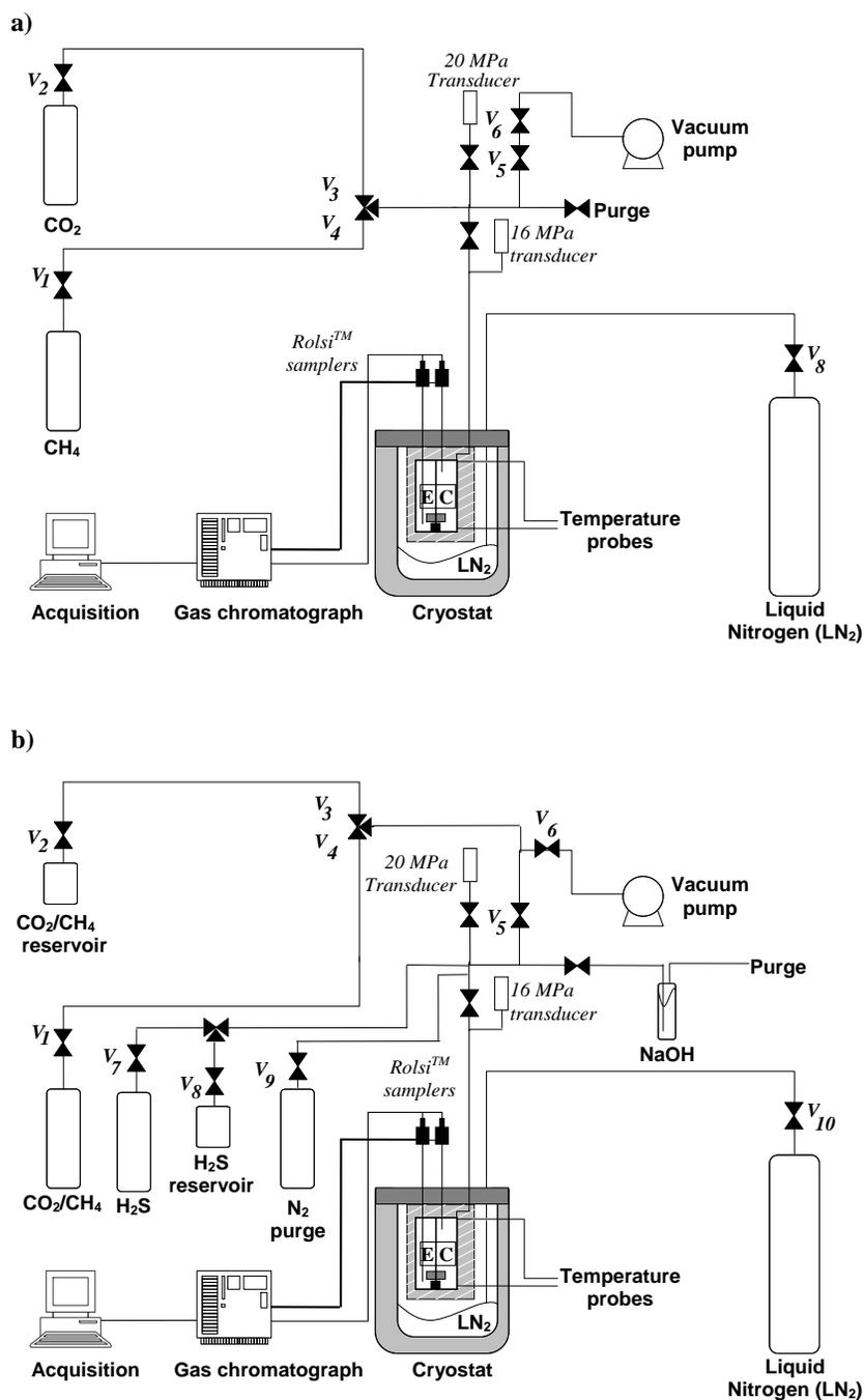
**Figure 1.** Flow diagram of the equipment used for a) TPxy solid apparition measurements for the CH<sub>4</sub>-CO<sub>2</sub> system and b) TPxy solid apparition measurements for the CH<sub>4</sub>-CO<sub>2</sub>-H<sub>2</sub>S system.
