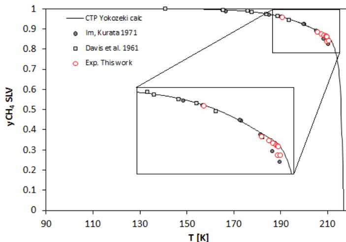
**Figure 5.** Comparison among literature data for the Ty SLV locus of the CH<sub>4</sub>-CO<sub>2</sub> mixture, experimental data obtained in this work and results obtained with the Yokozeki EoS [49] for SLV calculation.
