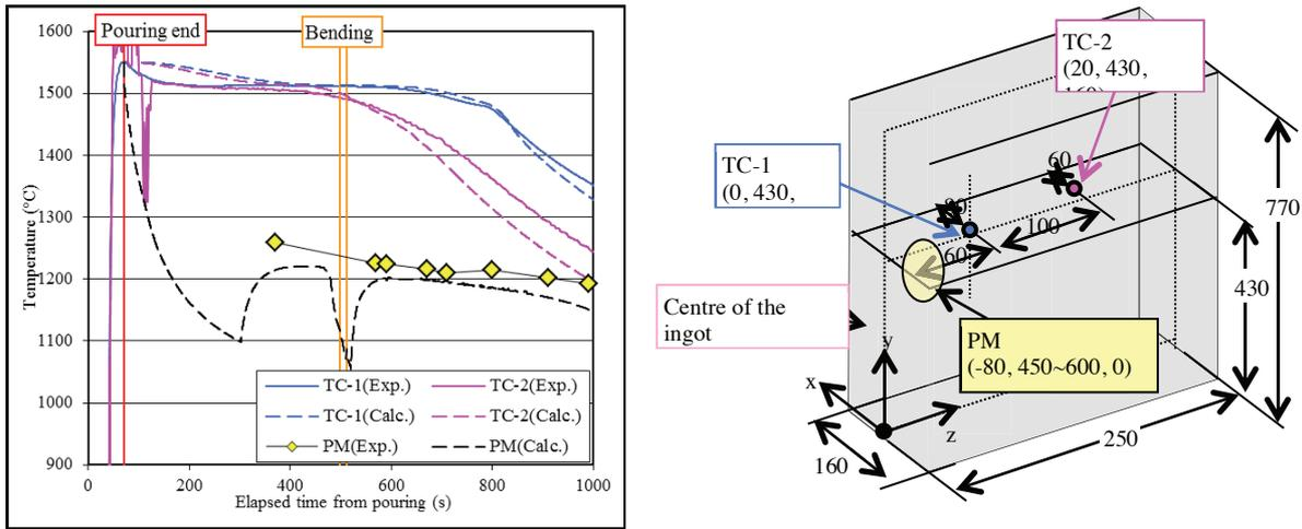
**Figure 2.** Comparison of temperature evolution in the ingot and schematic showing position of thermocouple TC-1 and TC-2 in the ingot, as well as the position at the ingot surface where pyrometer PM records the temperature after partial mold removal.
