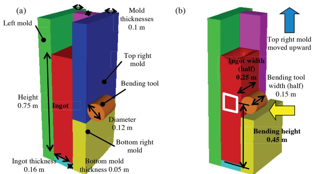
**Figure 1.** Schematic of the hot tearing experiment developed at Nippon Steel & Sumitomo Metal Corporation showing (a) initial state and (b) bending stage after partial mold removal. The configuration shown is half of the setup, considering symmetry with respect to the central transverse cut through the ingot, mold and bending tool domains.
