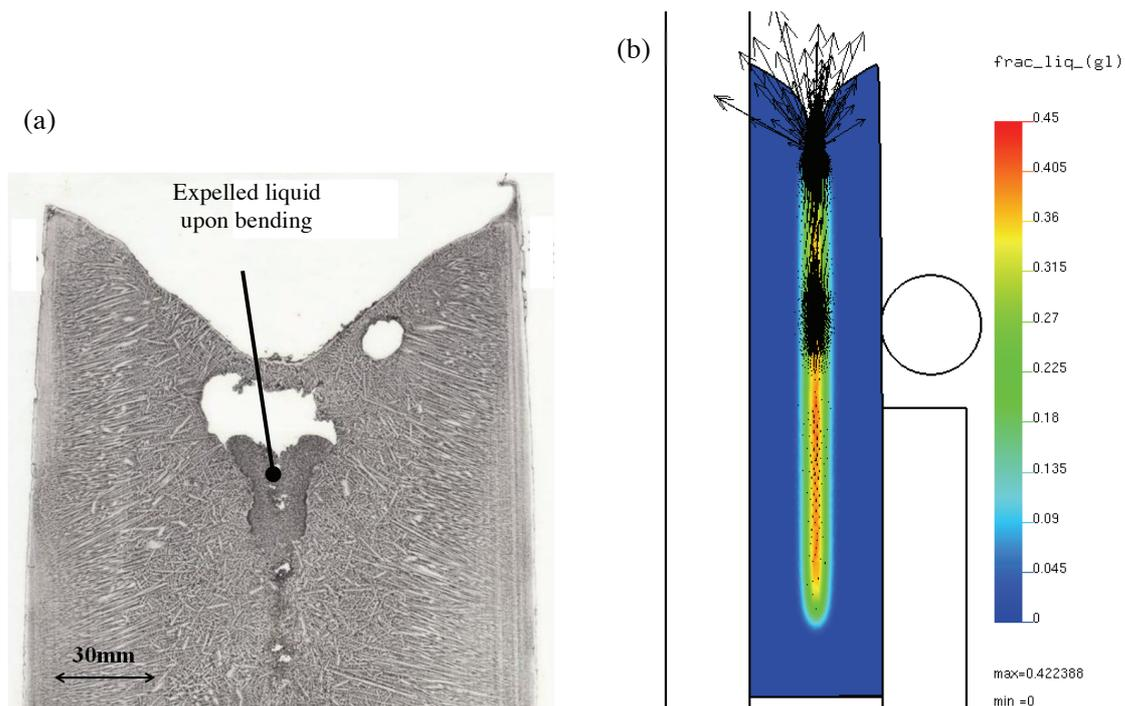
**Figure 6.** On the left, a micrograph of the ingot top for test N-1 shows the structure of the top ingot resulting from an expulsion of liquid upon bending: some liquid entered the primary shrinkage macrocavity. On the right, simulated relative velocity vectors in the liquid phase are superimposed on the liquid fraction field for trial N-1, showing the same phenomenon during bending.
