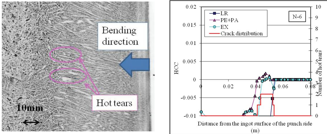
**Figure 4.** A micrograph of test N-6 and the comparison of the hot tearing sensitivity profile with the location of the hot tears in the bending region. Hot tearing sensitivity is calculated with the three microsegregation models.
