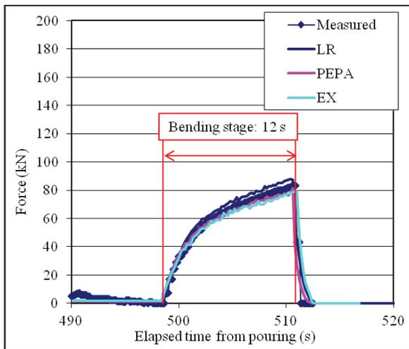
**Figure 3.** Force evolution during bending stage for trial N-4 deduced from measurements and from simulations using the three microsegregation models.
