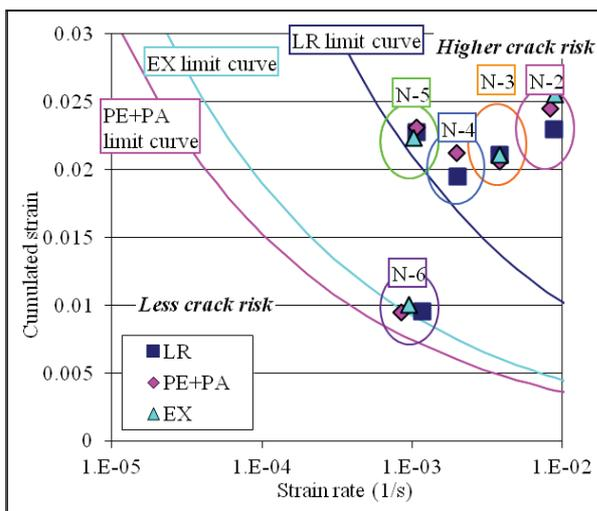
**Figure 5.** Computed cumulated strain,  $\int_{BTR} \hat{\epsilon} dt$ , as a function of the maximum perpendicular strain rate calculated when passing through the BTR. Values taken from the  $HCC_{WYSO}$  profile at the bending height, an example being shown in Figure 4b. The three continuous curves indicate the strain limit  $\hat{\epsilon}_C$  (Eq. 1).
