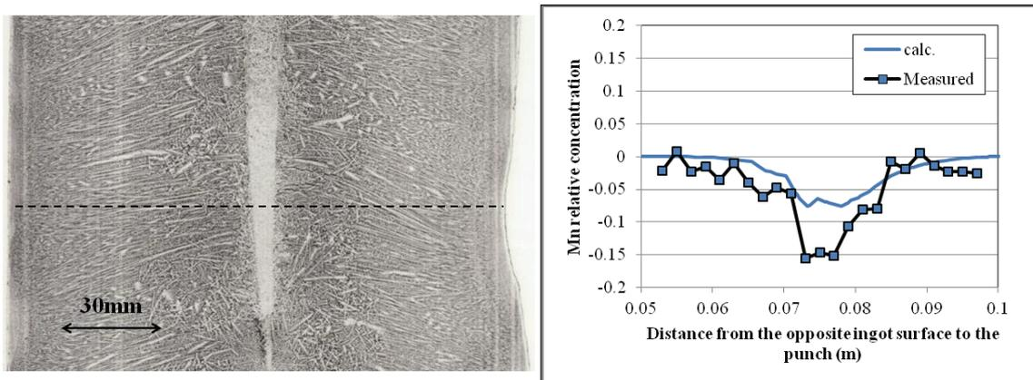
**Figure 7.** A micrograph of the ingot bending region for the test N-1 and comparison of Mn relative concentration profile at bending height with measurement result by means of EPMA. Simulation results show qualitative agreement with measurements.
