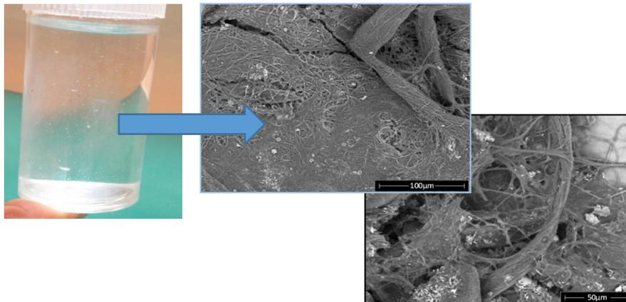
**Fig.8** Extractibles (small cell-walls components) removed during immersion observed by analysing the ageing water using an electronic microscope.
