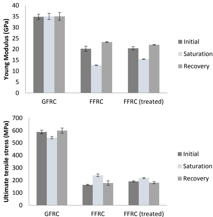
**Fig.6** Mechanical properties (Young's modulus and ultimate tensile stress) of glass and flax-fibre composites (untreated and silane treated flax fibre) before immersion, at saturation and after drying.
