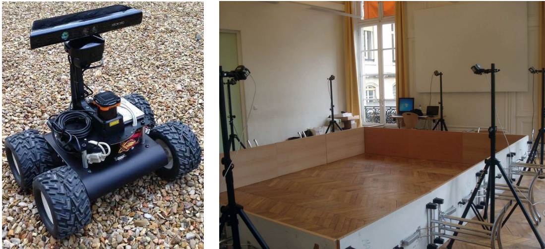
Fig. 1. The Wifibot Lab v4 Robot (left); Experiment area with motion-capture system (right)
