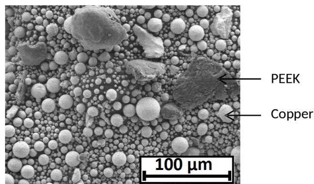
**Fig. 1.** SEM view of the powder mixture
