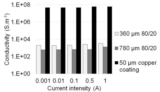
**Fig. 7.** Coatings conductivity
