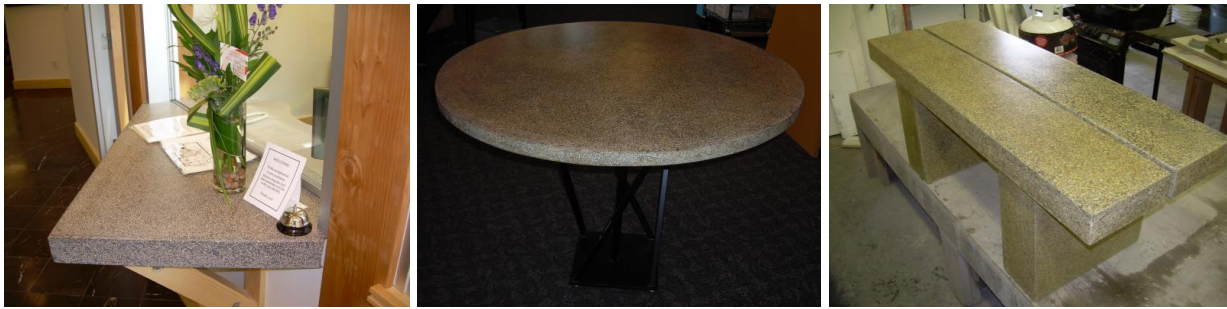
Figure 4. Various applications of mountain pine wood concretes [105]. With permission from Pasca, S & Hartley, ID 2012, 'Beetlecrete – An attractive solution to mountain pine beetle epidemic', Proceedings of International Inorganic-Bonded Fiber Composites Conference (IIBCC 2012), 10-14 September, 2012, Acton, Australia. (Available from: www.proceedings.com , Item #20276)
