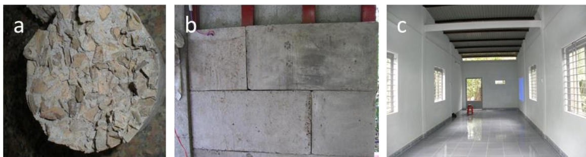
Figure 3. Coconut reinforced concretes: a) a concrete block, b) the concrete panels and c) the house built from them (with permission of Nguyen Tan Khoa and his supervisor (Dr. Le Anh Tuan) [104].
