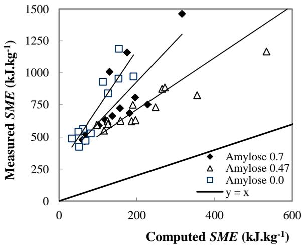
Figure 2. Validation of Ludovic® simulation for  $SME$
