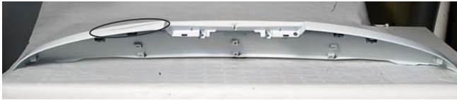
Figure 2. Bottom view of a spoiler (the defective zone is bordered)
