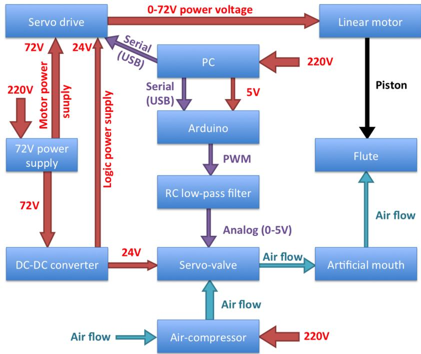
Figure 1: Synoptic diagram of the system — Red stands for power supply, purple for logic and cyan for air flow.
