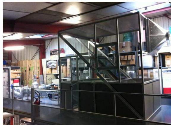
Figure 1: Test bench: aerodynamic chamber and regulated ventilator
