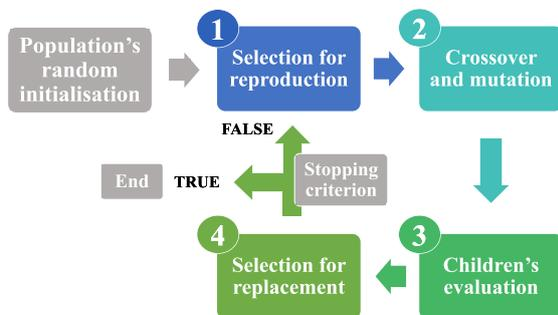
Figure 1 Illustration of the genetic algorithm process
