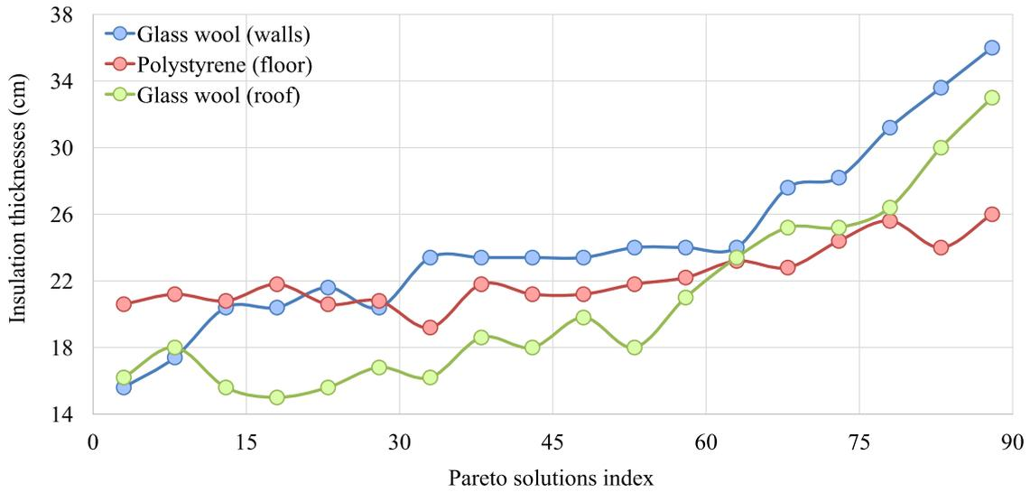
Figure 8 Evolution of the insulation thicknesses for decreasing GHG emissions (Pareto solutions)
