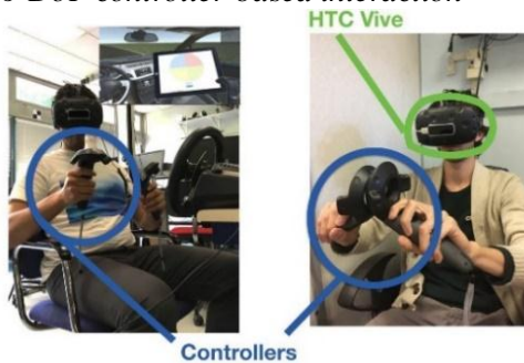
Fig. 3 – 6-DoF controller-based interaction
