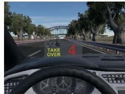
Fig. 5 – Take Over Request displayed on the HUD
