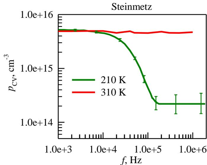
Fig. 8 Apparent concentration vs. frequency for Steinmetz sample;  $T = 210$  and  $310$  K. Error bars are shown
