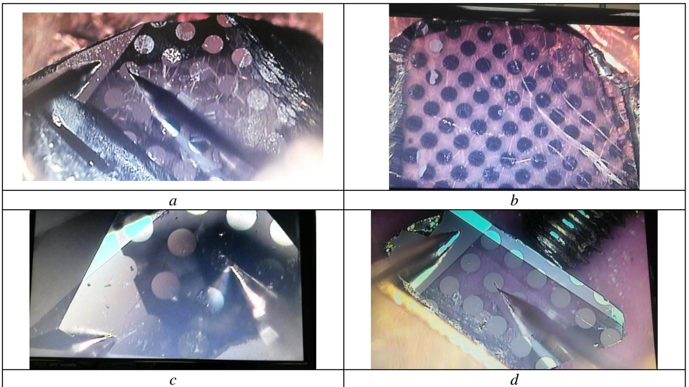
Fig.2 View of investigated samples with sputtered contacts and measuring probes: *a* – Apollo Blue, *b* – Diamond 111, *c* – Blue Pear, *d* – Steinmetz
