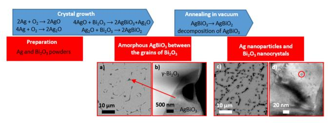
Figure 5 Silver evolution mechanism in  $Bi_2O_3$ -Ag system, starting from the crystal growth through the post-growth annealing processes. *Blue arrows* represent processes, *red rectangles*—the resulting micro-/nanostructure. SEM pictures of the
