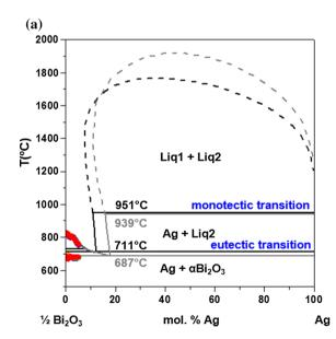
Figure 1 Eutectic phase diagram of  $Bi_2O_3$ -Ag system. Adapted with permission from Wiley. Liquidus and solidus curves (*dots*) for  $Bi_2O_3$ -Ag mixtures measured in atmospheres with different
