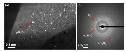
**Figure 3** Decomposition of the amorphous AgBiO<sub>3</sub> phase under electron beam irradiation into nanocrystalline  $\gamma$ -Bi<sub>2</sub>O<sub>3</sub> precipitates and metallic silver to **a**  $\gamma$ -Bi<sub>2</sub>O<sub>3</sub> seen as bright grains in the dark-
