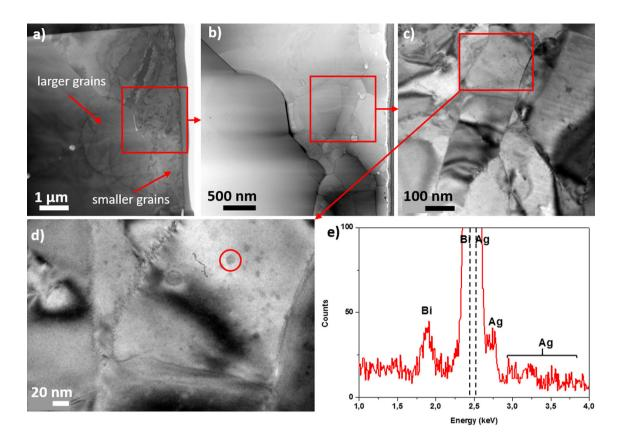
**Figure 4** Structural analysis of the annealed-in-vacuum  $Bi_2O_3$ -Ag eutectic material. **a**–**c** Progressive zooms by HAADF showing the various scales of the structure with the smaller and larger grains
