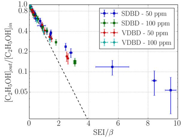
Fig. 6. Ethanol residual concentration as a function of the ratio  $SEI/\beta$  for SDBD and VDBD at two inlet concentrations: 50 ppm and 100 ppm. Error bars correspond to a 95% confidence interval. The dashed line corresponds to the  $\exp(-SEI/\beta)$  curve.
