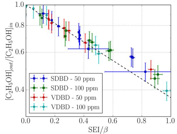
Fig. 7. Ethanol residual concentration as a function of the ratio  $SEI/\beta$  for SDBD and VDBD at two inlet concentrations: 50 ppm and 100 ppm and  $SEI/\beta < 1.0$ . Error bars correspond to a 95% confidence interval. The dashed line corresponds to the  $\exp(-SEI/\beta)$  curve.
