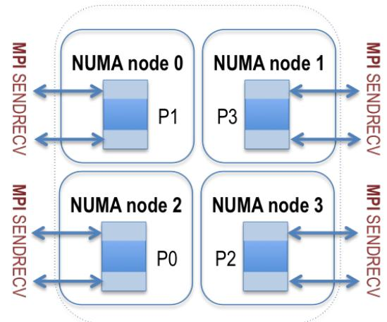
Fig. 6. MPI Layout on a Manycore Node
