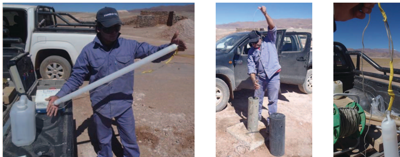
FIG 2 – Capturing brine at chosen depths by using bailers.
