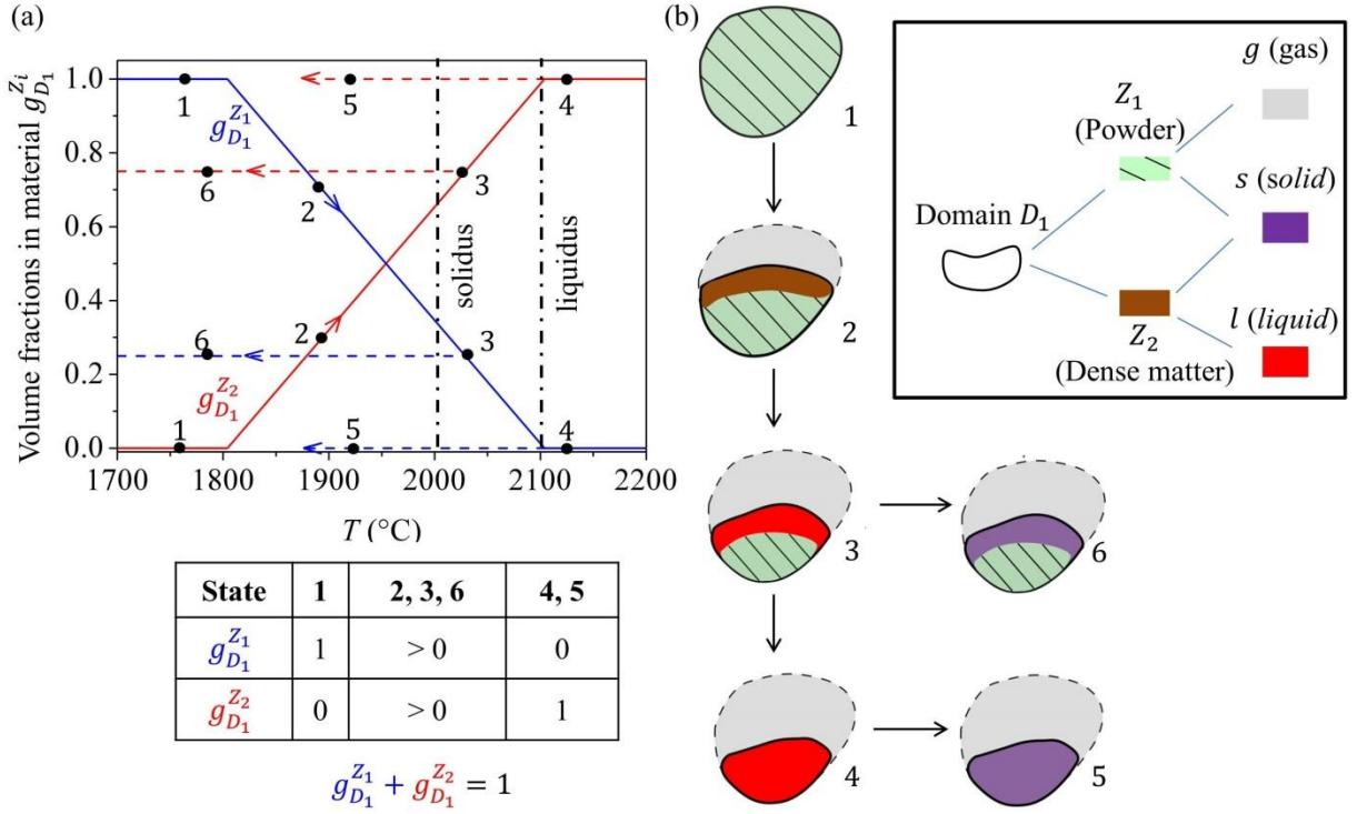
Figure 4: One-way transformation from powder (zone  $Z_1$ ) to dense matter (zone  $Z_2$ ) with (a) volume fractions as a function of temperature in domain  $D_1$  and (b) illustration of possible distribution of zones and phases depending on the maximum heating temperature reached during the thermal history, (state 5) above and (state 6) below the melting temperature of the dense matter. Other states represent intermediate status of domain  $D_1$  during the transformation path.
