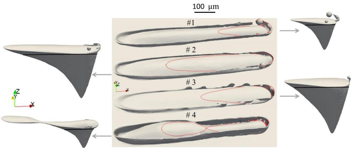
Figure 8: Simulated bead shape (center) and melt pool shape (two sides) for cases 1~4 at  $t = 3$  ms. Gas and powder are removed and the red contour indicates the melt pool. The skirt around the bead corresponds to powder partially melted and solidified. The black line is the powder/substrate boundary.
