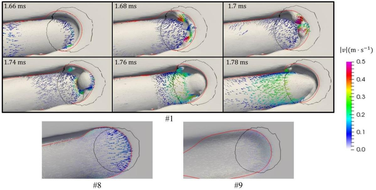
Figure 13: Comparison of melt pool of cases 1, 8 and 9 with different value of the surface tension. The melt pool (red, iso-contour of liquidus) and the laser spot (black contour) with  $R_L = 35 \mu\text{m}$  are highlighted. The surface in cases 8 and 9 is drawn with transparency in order to better show the velocity field as the fluid flows is principally developed below the surface.
