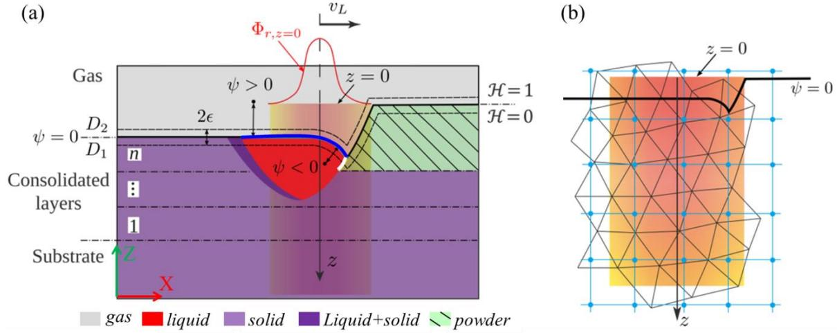
Figure 2: Schematics of (a) modeling of additive manufacturing (AM) by selective laser melting (SLM) with the level set (LS) method used to track the isovalue  $\psi = 0$  of the signed distance function to the interface and (b) numerical implementation of the heat source (FE mesh in black, regular grid in blue).
