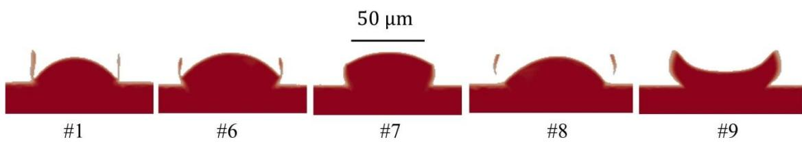
Figure 12: Transversal cross sections at  $X = 0.5$  mm,  $t = 2$  ms of case 1, 6, 7, 8 and 9. Gas and powder are removed.
