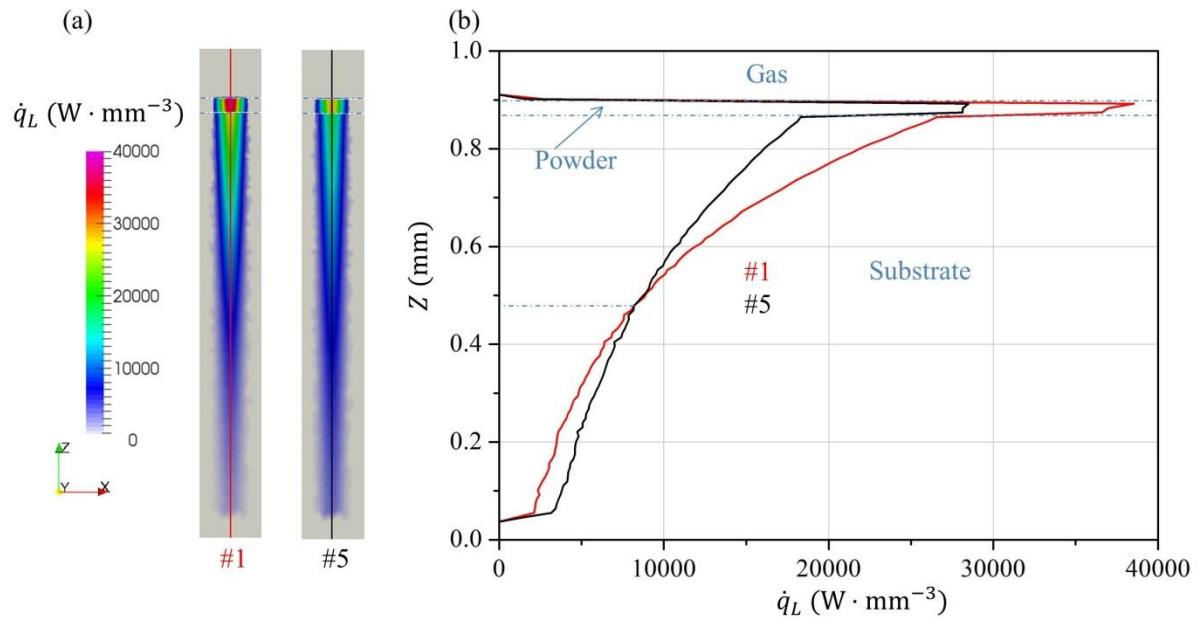
Figure 11: (a) Heat source distribution and (b) profile along laser axe of case 1 (red) and 5 (black) with different absorption coefficient at  $t = 4 \mu\text{s}$  (corresponding to 24.6% of  $P_L(1 - R)$  imposed).
