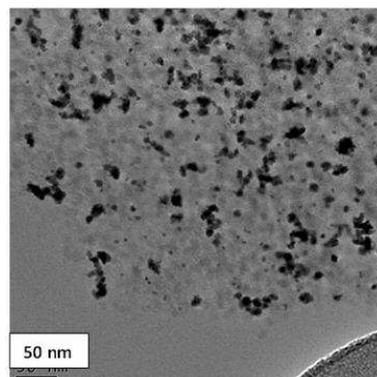
Figure 1. TEM pictures of the Pt-CA electrocatalyst.
