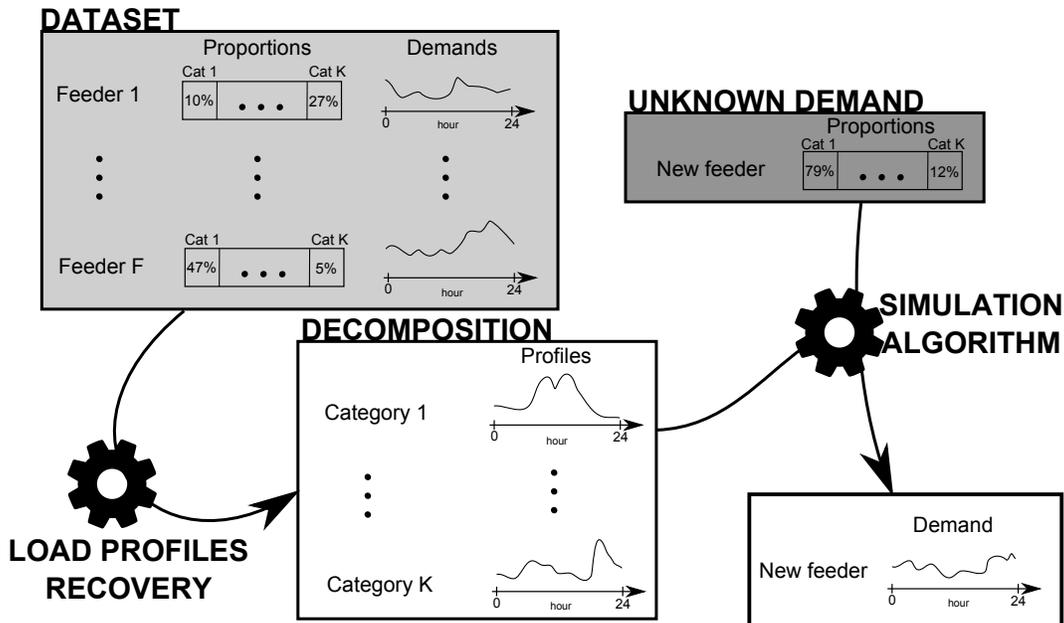
Figure 1: Diagram detailing the method. A dataset of  $F$  feeder measurements is used to find the  $K$  category profiles. Once the load profiles recovery is operated, a new feeder whose category distribution is known can be run through the simulation algorithm in order to obtain its expected demand.
