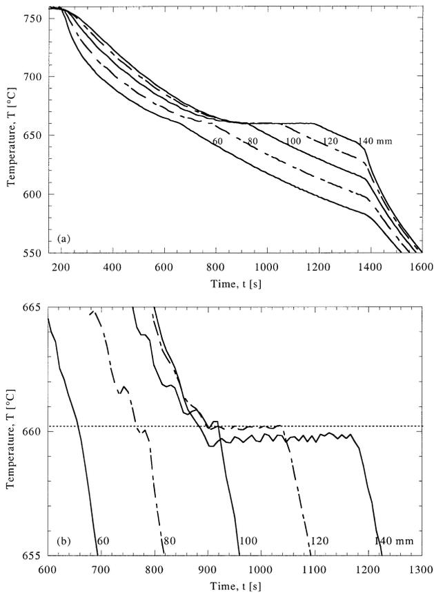
**Fig. 3.** Recorded cooling curves at different heights from the bottom of the ingot in the 99.99 wt% Al ingot shown in Fig. 1(a). Figure 3(b) is a magnification of Fig. 3(a) made in a narrow range of temperature surrounding the melting temperature (horizontal dotted line at 660.2°C).
