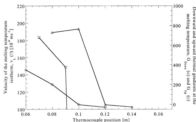
Fig. 5. Average velocities of the melting temperature isotherm,  $v_L$ , calculated between two thermocouples (left scale) and thermal gradients ahead,  $G_{\text{Up}}$ , and below,  $G_{\text{Down}}$ , the position of the thermocouples at the time they are reached by the melting temperature (right scale), using the experimental and simulated cooling curves recorded in the 99.99 wt% Al ingot (Fig. 3).
