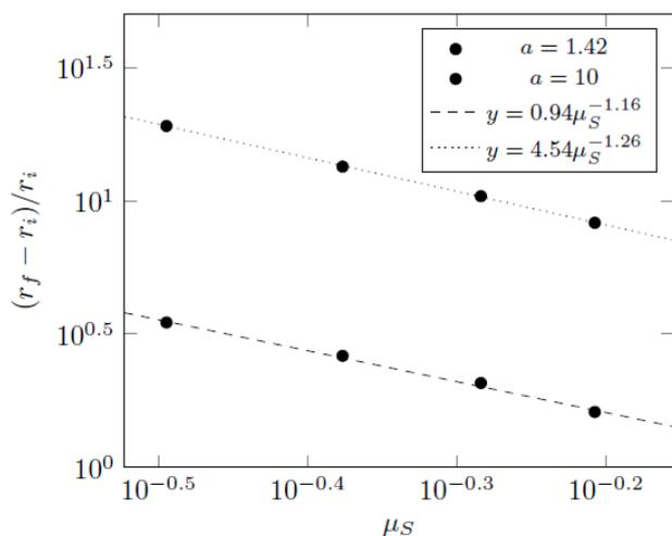
**Fig. 5.** Variation of relative spreading with quasi-static friction coefficient for different aspect ratios
