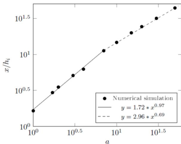
**Fig. 3.** Relative spreading distance vs. initial aspect ratio for 2D computations
