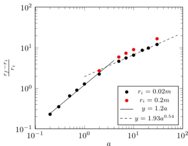
**Fig. 4.** Relative spreading distance vs. initial aspect ratio for 3D computations – Influence on the initial column height (for each value of aspect ratio  $a$ , two different radii give two different column heights)
