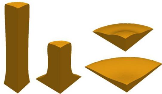
**Fig. 1.**  $\mu(I)$  computation of the shape of a granular column at time  $t = 20\%$ ,  $40\%$ ,  $60\%$  and  $80\%$  of total collapse, for an initial ratio  $a=7$ ; rheological parameters were taken from [5]
