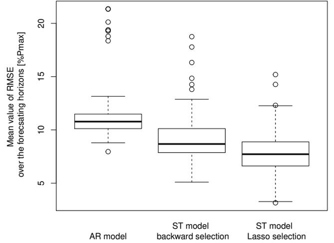
Fig. 8. Data set  $d_2$ : Distribution of the mean value (over the 6-hour prediction horizon) of RMSE for the reference model, the spatio-temporal model (ST) with backward selection, and the spatio-temporal model with Lasso selection.
