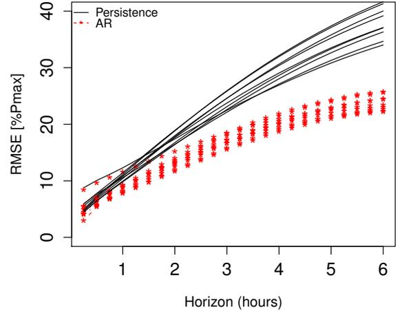
Fig. 3. Data set  $d_1$ : Comparison of the normalized RMSE of AR and persistence models over the testing set. Solid and dotted lines represent respectively the performance of persistence AR models. The forecast time step is 15 min.
