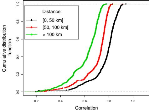
Fig. 2. Data set  $d_2$ : Cumulative distribution function (CDF) of the cross-correlation between the lagged production series. Green, red and black CDFs respectively described three classes of distance between the power plants.
