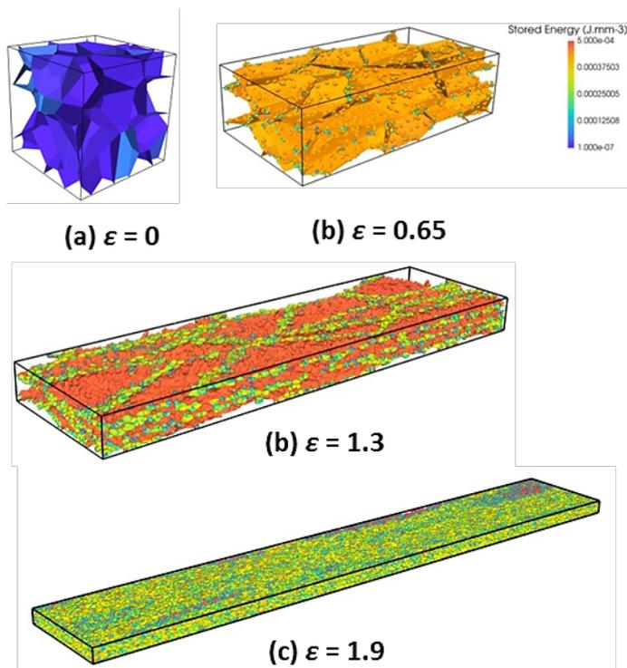
Figure 1. Simulation of a channel-die compression of the 304L steel at 1000°C and at a strain rate of 0.01s<sup>-1</sup>. Four different instants are represented: (a)  $\varepsilon = 0$ , (b)  $\varepsilon = 0.65$ , (c)  $\varepsilon = 1.3$ , (d)  $\varepsilon = 1.9$ . The initial number of grains is 64 and the final number of grains is around 50.000.
