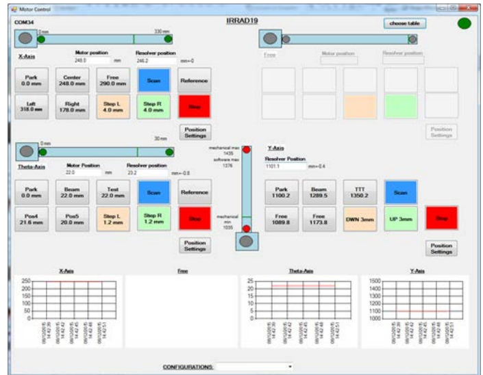
Fig. 3. User interface of the IRRAD table control system.
