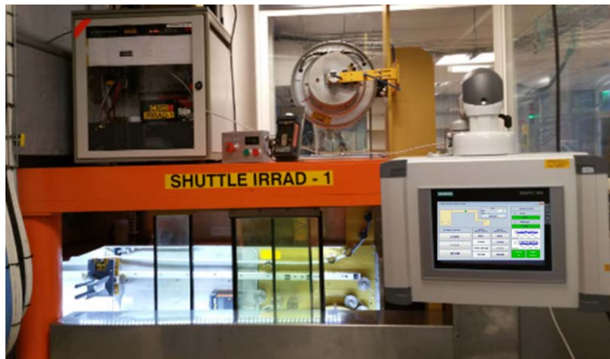
Fig. 5. LOAD position of the shuttle IRRAD1, outside the control room of IRRAD. The users' interface depicted in Fig. 6 is also visible here.
