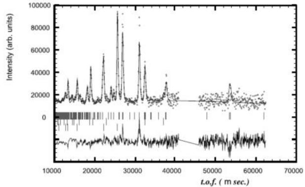
**Fig. 8.** Observed (crosses), calculated (continuous line), and difference (bottom) Rietveld ND profiles at 480 °C. The rows of tick marks give the positions of the allowed in  $Pnma$  space group Bragg reflections for the main phase of BCY15 (upper) and the minor contribution of Al foil (middle) and Cu heater (lower). The affected region of the pattern because of experimental geometry is excluded from the refinement.
