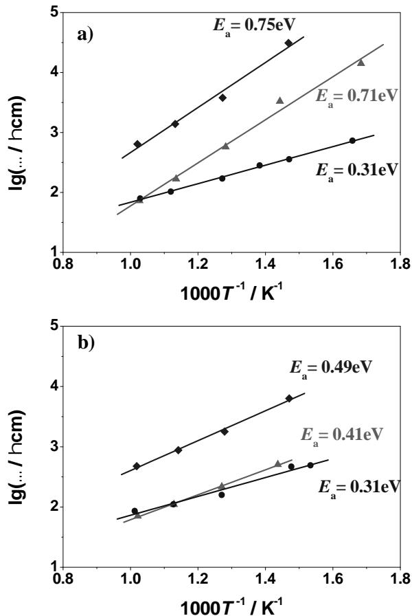
**Fig. 13.** Arrhenius plots of BCY15 samples with different porosity measured in dry air (a) and wet hydrogen (b): (◆) - sample 5 (47% porosity), (▲) - sample 4 (35% porosity), (●) - sample 3 (27% porosity).
