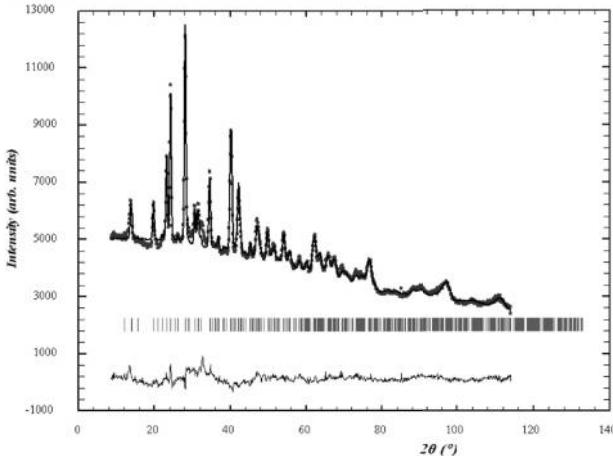
**Fig. 10.** Observed (crosses), calculated (continuous line), and difference (bottom) NPD Rietveld profiles of BCY15 protonated powder at 295 K. The row of tick marks gives the positions of the allowed Bragg reflections.
