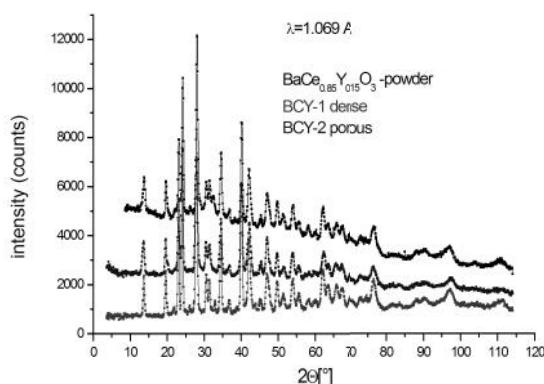
**Fig. 4.** ND patterns of BaCe<sub>0.85</sub>Y<sub>0.15</sub>O<sub>3</sub>- based samples at 295 K: a) constant wavelength ( $\lambda = 1.069 \text{ \AA}$ ) pattern. The sample denoted as powder was kept for three days in moist air; b) TOF patterns: 1 (dense), 2 (porous), 3 (powder). The patterns are vertically shifted to improve visibility.
