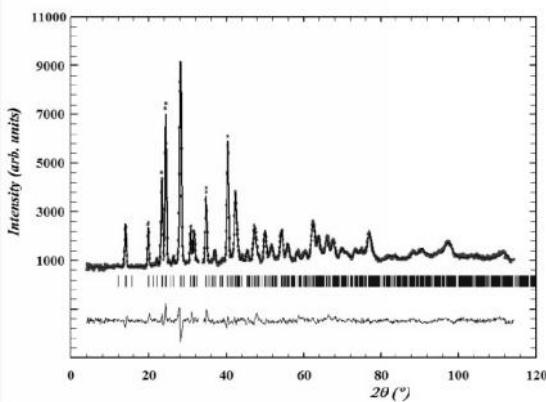
**Fig. 5.** Observed (crosses), calculated (continuous line), and difference (bottom) Rietveld ND profiles of milled material of dense BCY15 pellet at 295 K. The row of tick marks gives the positions of the allowed Bragg reflections.
