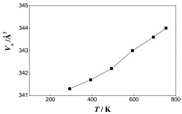
**Fig. 9.** Temperature dependence of unit cell volume  $V_o$  of BCY15 pellet of 13% porosity.
