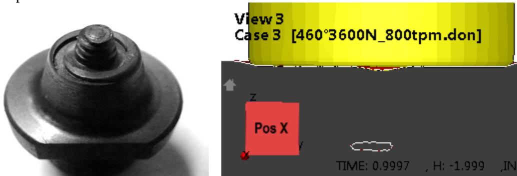
**Figure 1:** (a) Conical tool with threaded pin and scrolled shoulder (b) Development of worn hole defect in the simulation that perfectly corresponds with macrographs from FSW trials [3].
