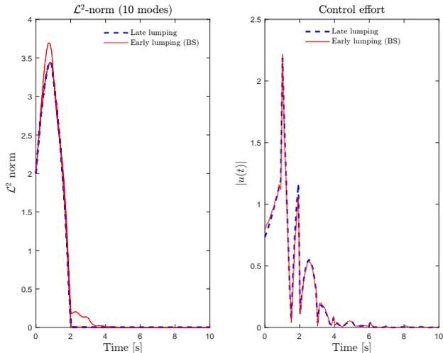
Fig. 8. Time evolution of the  $\mathcal{L}^2$ -norm and of the control efforts for different controllers (system (51)-(53),  $N=40$ ,  $M=10$ )
