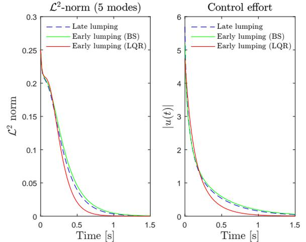
Fig. 2. Time evolution of the  $\mathcal{L}^2$ -norm and of the control efforts for different controllers (heat equation,  $N=30$ ,  $M=5$ )
