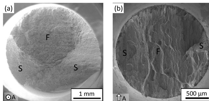
Figure 7. Macroscopic view of typical fracture surfaces of smooth specimens after creep (a) along AD (gauge diameter 4 mm, applied stress 350 MPa, minimum creep rate  $9.4 \times 10^{-10} \text{ s}^{-1}$ , creep lifetime 417h), and (b) along RD (gauge diameter 2 mm, applied stress 250 MPa, minimum creep rate  $1.3 \times 10^{-8} \text{ s}^{-1}$ , creep lifetime 140 h). F: flat fracture; S: slant fracture
