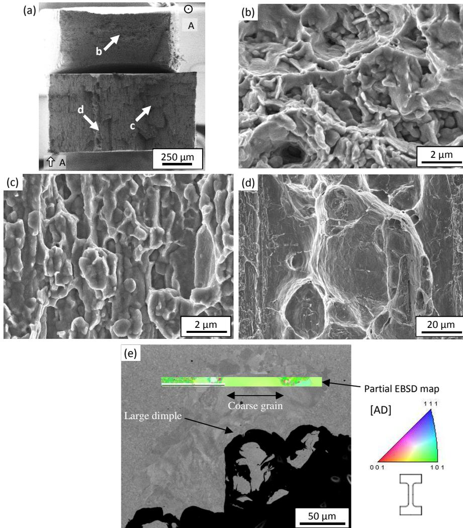
Figure 4. (a) Global view of fracture surfaces of AD and RD FT specimens, pulled at 650°C –  $7 \times 10^{-4} \text{ s}^{-1}$ , (b) enlarged view of the fracture surface of the AD specimen, (c) and (d) enlarged views of the fracture surface of the RD specimen. (e) cross section under large dimples with superimposed partial EBSD map (color code: orientation of AD in the crystal frame)
