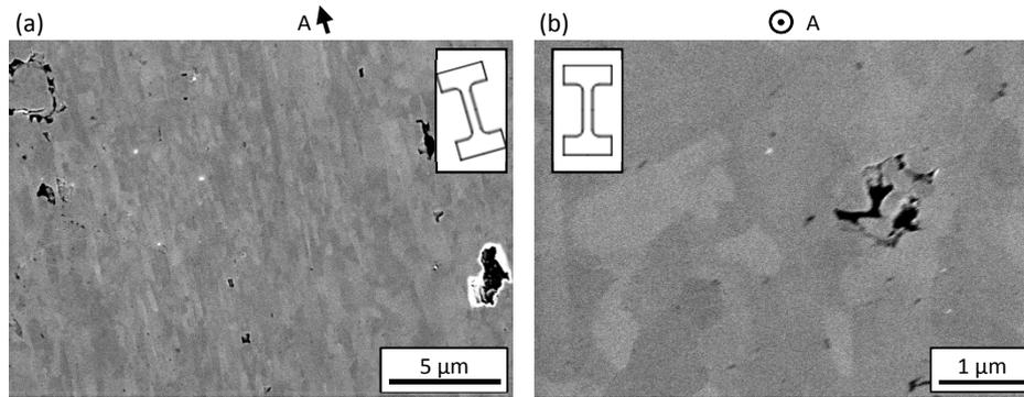
Figure 6. SEM observations of cross sections of FT specimens pulled at  $650^{\circ}\text{C}$  at  $7 \times 10^{-4} \text{ s}^{-1}$  along (a) AD and (b) RD.
