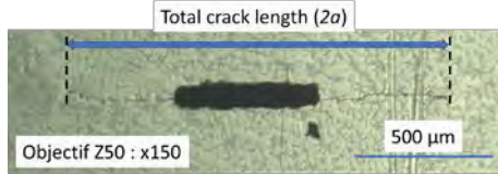
Fig. 14. Crack growth image analysis
