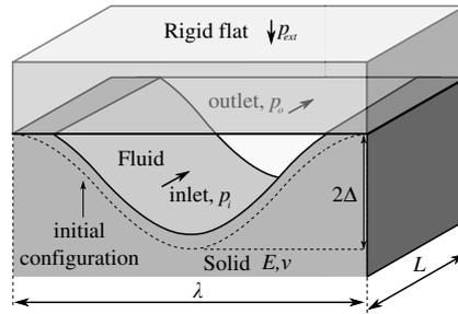
FIGURE 5 – Fluid flow through a periodic wavy contact interface.
