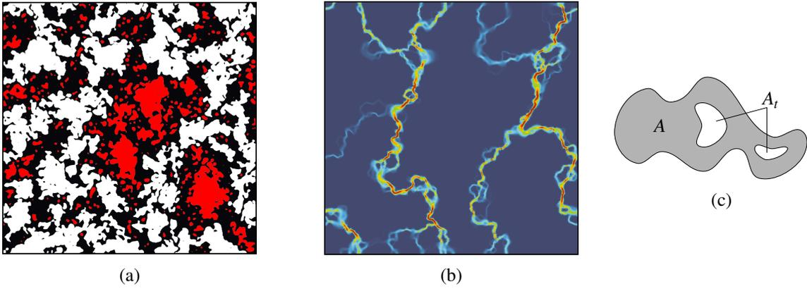
FIGURE 1 – (a) Morphology of contact patches for the contact of a 3D body with a rigid plane : black is the contact area, white is out of contact and red is "trapped". (b) Incompressible fluid flow through the same contact interface (color represents the flow intensity). (c) An example of non-simply connected contact patch :  $A$  is the contact area,  $A_r$  is out-of-contact (trapped) area.
