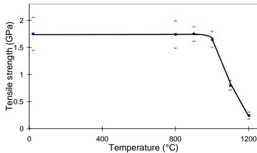
Fig.8: Tensile strength at a constant strain rate of  $6 \cdot 10^{-5}$ /s as a function of temperature
