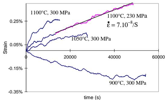
Fig.12: Creep curves of monofilaments
