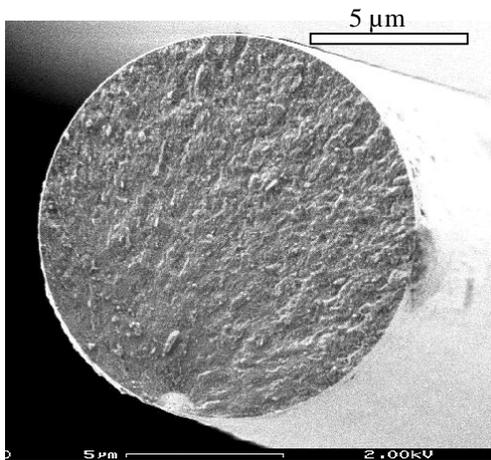
Fig.1: SEM micrograph of the N720 fibre
