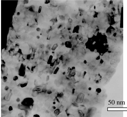
Fig.5: Microstructure after a heat treatment of 4 hours at 1400°C
