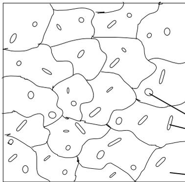
As schematised on Fig.14 the Nextel 720 fibre is composed of aggregates of mullite composed of grains separating by low angle disorientations and enclosing round or elongated  $\alpha$ -alumina grains. The elongated alumina grains have got aspect ratios of up to 6 and they are mainly orientated in the fibre axis direction.
