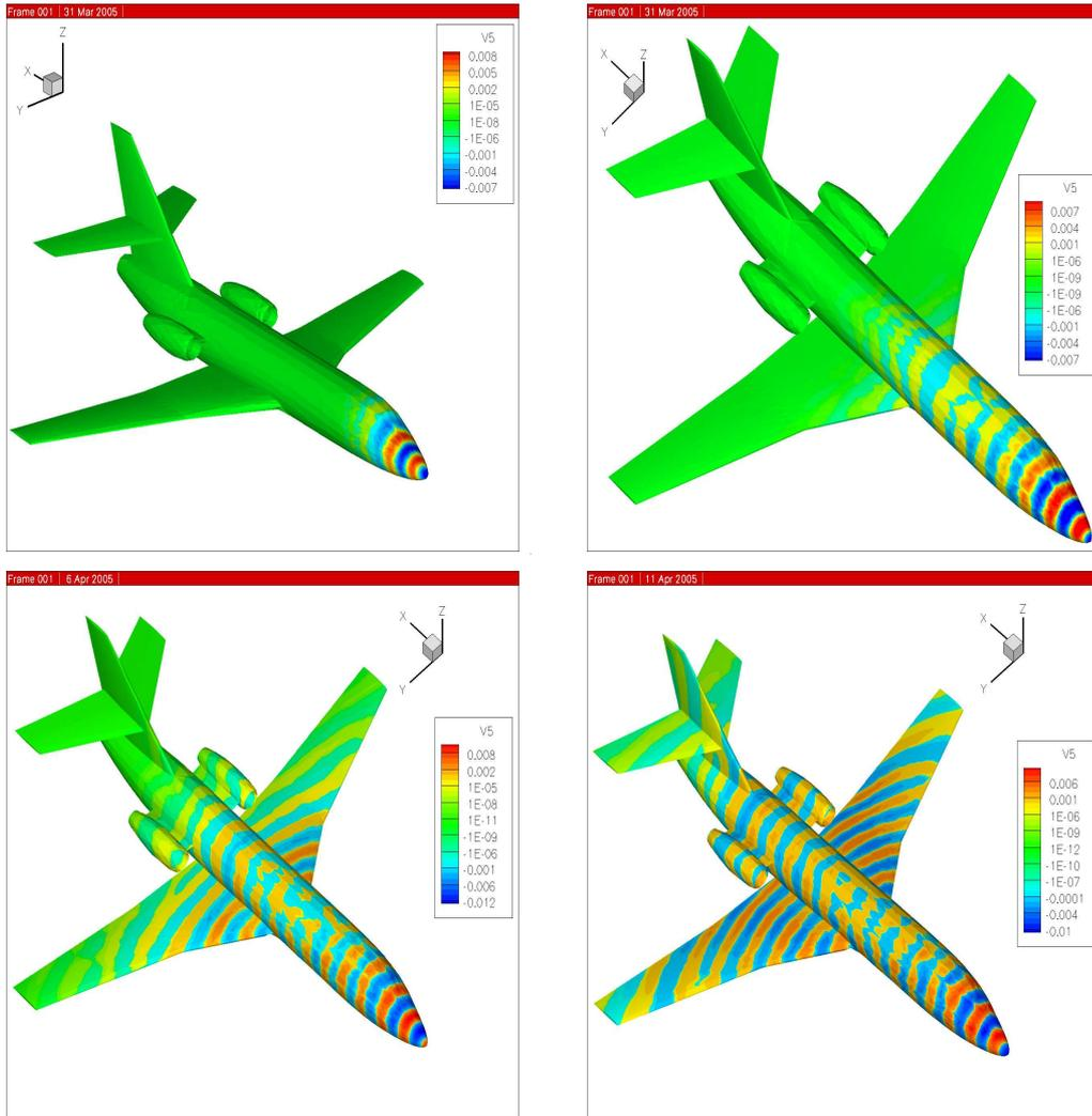
Figure 7: Surface contours for  $\delta p$  (times  $t = 1s$ ,  $t = 2s$ ,  $t = 2.7s$ ,  $t = 3.5s$ ).
