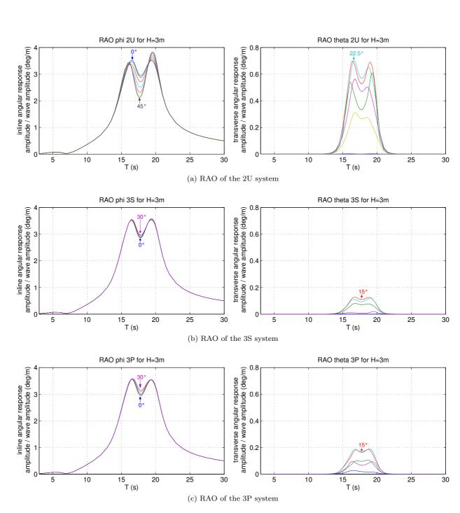
Figure 8: RAO of an arrangement of multiple TLCDs (a) and variants of TLMCDs ((b) and (c)) for different wave incidences of a 3 m monochromatic wave
