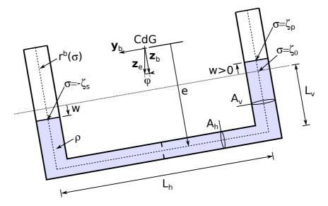
Figure 3: Scheme of a single TLCD illustrating the main variables
