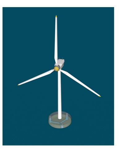
Figure 2: Illustration of the float with a 3S TLMCD  $\,$
