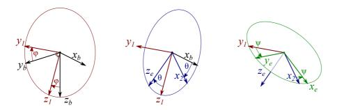
Figure 4: Orientation of  $\mathcal{R}_b$  with respect to  $\mathcal{R}_e$
