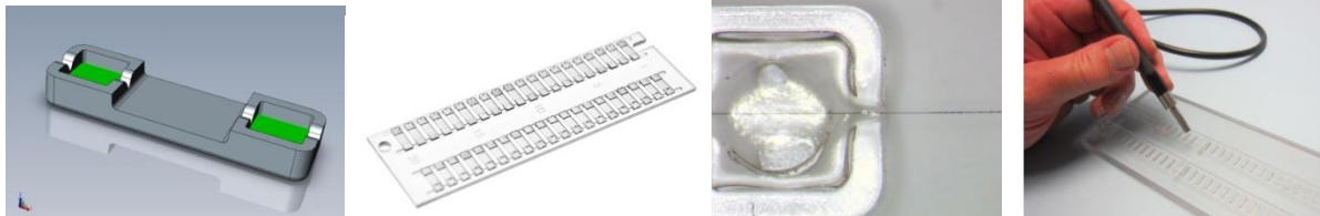
Figure 2: (a) Plastic tab for holding a fibre (b) 20 sample cassette (c) Wells in tabs for accurate gauge lengths (d) UV curing of adhesives
